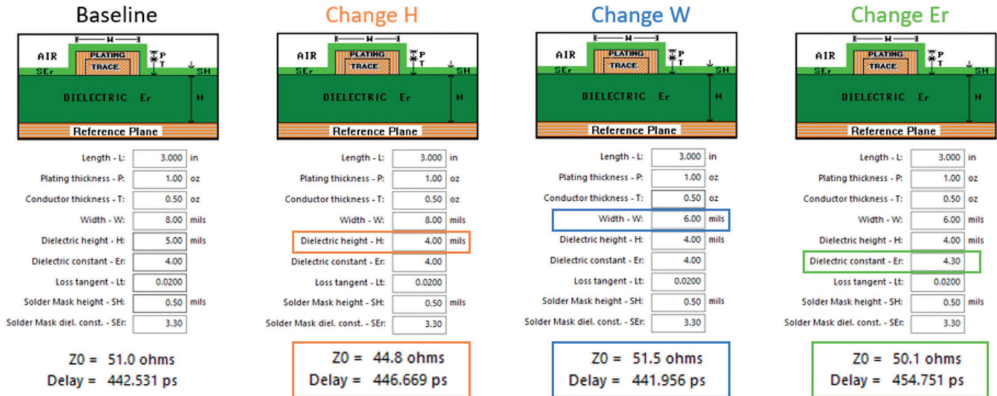
Figure 23. PCB microstrip examples.
