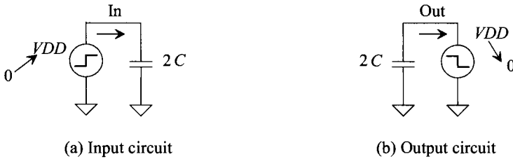
Figure 10.3 Splitting the capacitor in Fig. 10.2 up into two equivalent capacitors for developing a model.
