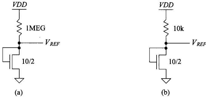
Figure 23.3 Resistor-MOSFET references used in Ex. 23.1
