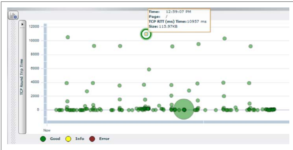
Figure 10-1. A scatterplot of page requests over time in Coradiant’s TrueSight, showing relative TCP round-trip time
