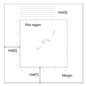
Graphics parameters controlling figure layout include:
