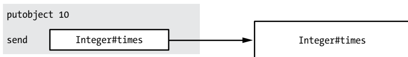
Figure 6-9: The inline cache saves the result of method lookup next to the send instruction that needs to call the method.
