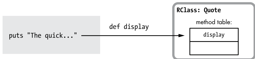
Figure 9-3: Ruby adds new methods to the method table for the target class.
